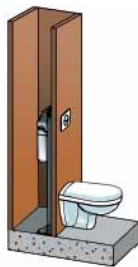
Installation en gaine technique
