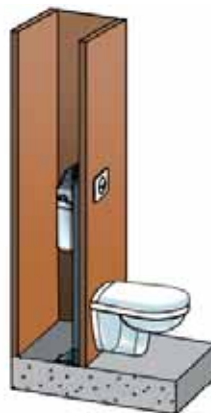
Installation en gaine technique
